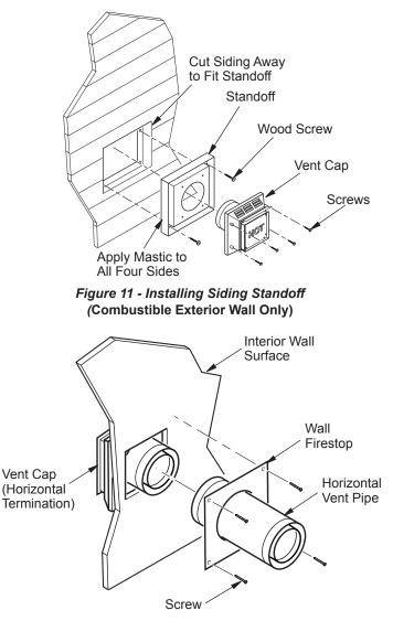
Figure 12 - Connecting Vent Cap with Horizontal Vent Pipe
